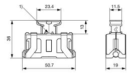
1) Position for optional terminal marking (terminal block width: 5.2 mm, lettering field: 4.6x5.1 mm, e.g. item 0818153 from Phoenix Contact)
